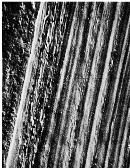
Fig. 7. Scanning electron micrographs of peeled surface of fiber E ( \times 5700 ) (peeling was done very near to the fiber surface).
